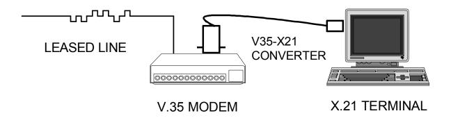
The maximum tested data rate is 6Mbps using the supplied 6 foot shielded data cable. Shorter and longer data cables will effect the V35-X21 Interface Converter data rate. The chart below indicates the interface control signals supported by the V35-X21.
